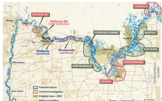
Figure 2: Salt Interception Scheme (SIS) in South Australia, to collect highly saline ground water before entering into the Murray River (source DWLBC, 2008).
