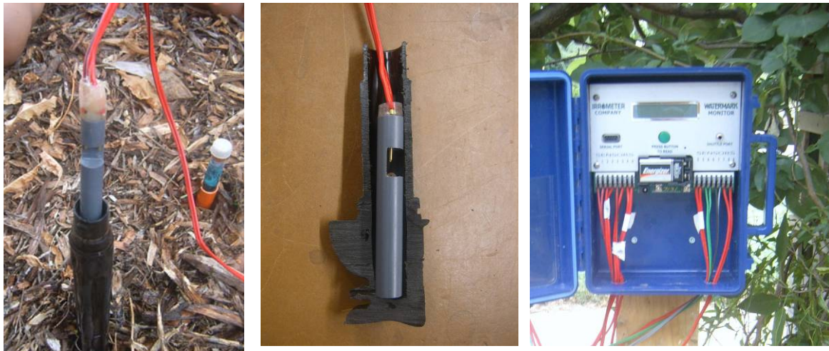
Figure 1. The conductivity probe being lowered into the float housing of a WFD (left) the position of the electrode in the base piece of the WFD (centre) and the 8 channel Irrrometer logger with in field display (right).
