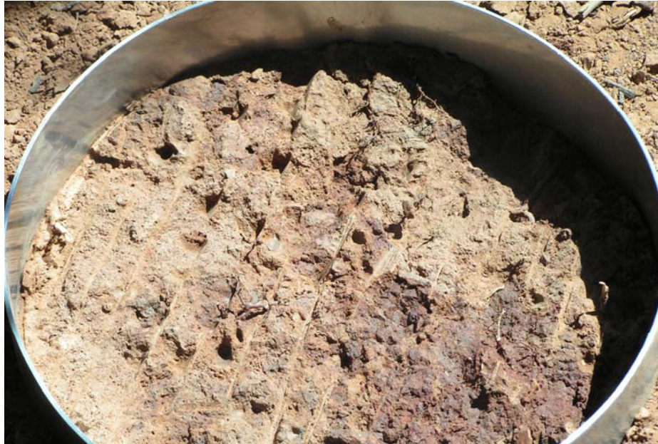
Figure 1: A subsoil surface prepared for infiltration measurements; macropores and roots are clearly visible.
